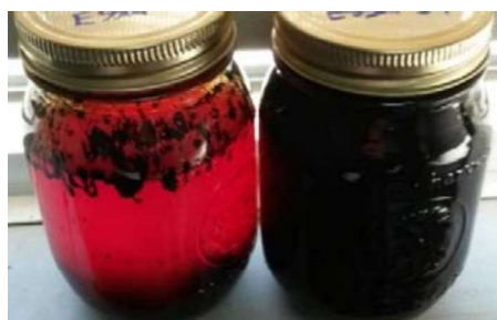
Figure 2: Wood vinegar (left) and bio-crude oil (right)
